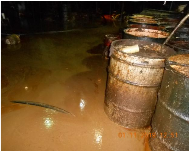
Improper storage of LIB (biodiesel)
