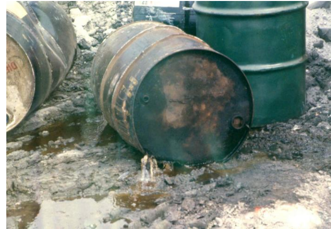
HW drum leaking to the ground
